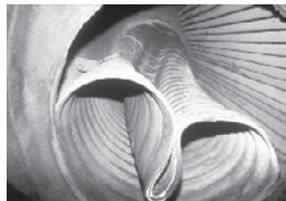
*A classic case of boiler damage, caused by the use of a low-level alarm operating with a float.*
